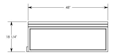
NOTE: FOR NON-STANDARD LENGTHS THE CHANNEL WILL BE SOLID BOTTOM AND DESIGNATED WITH ITS CORRESPONDING LENGTH MEASUREMENT. IE: 805016F 32"
