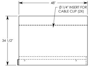
**NOTE 1:** FOR NON-STANDARD LENGTHS THE CHANNEL WILL BE SOLID BOTTOM AND DESIGNATED WITH ITS CORRESPONDING LENGTH MEASUREMENT. IE: 805024HT 32"
