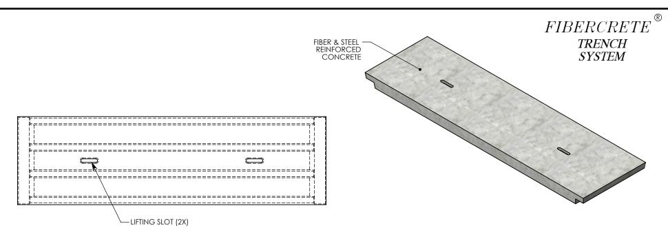
COVER ASSEMBLES ONTO 50" INSIDE WIDTH PEDESTRIAN RATED CONCAST **PT** CHANNEL.
