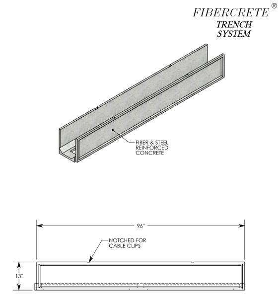
NOTE: FOR NON-STANDARD LENGTHS THE CHANNEL WILL BE SOLID BOTTOM AND DESIGNATED WITH ITS CORRESPONDING LENGTH MEASUREMENT. IE: 8810 32"
