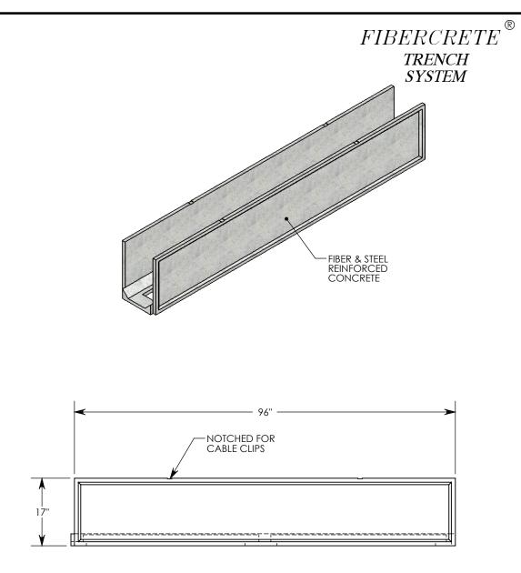
NOTE: FOR NON-STANDARD LENGTHS THE CHANNEL WILL BE SOLID BOTTOM AND DESIGNATED WITH ITS CORRESPONDING LENGTH MEASUREMENT. IE: 881016 32"
