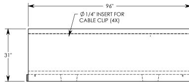
**NOTE 1:** FOR NON-STANDARD LENGTHS THE CHANNEL WILL BE SOLID BOTTOM AND DESIGNATED WITH ITS CORRESPONDING LENGTH MEASUREMENT. IE: 801024HT3 32"
