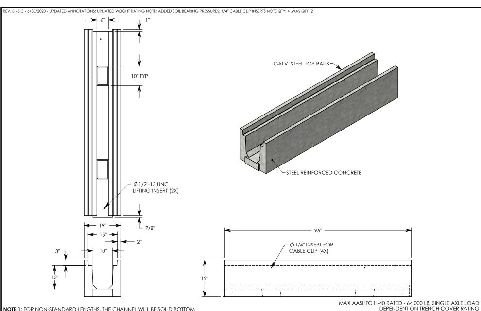
**NOTE 1:** FOR NON-STANDARD LENGTHS, THE CHANNEL WILL BE SOLID BOTTOM AND DESIGNATED WITH ITS CORRESPONDING LENGTH MEASUREMENT. IE: 8010HT3 72"
