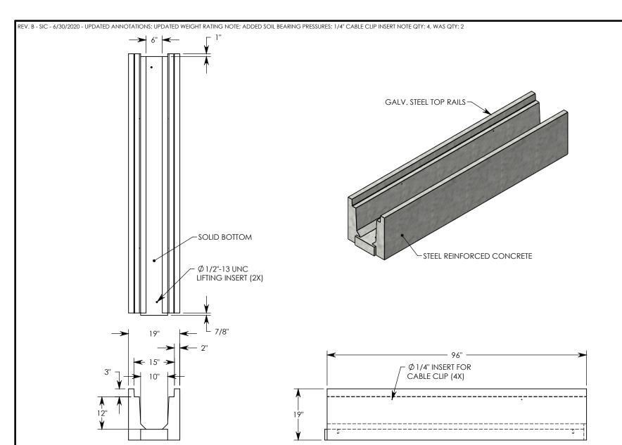
**NOTE 1:** FOR NON-STANDARD LENGTHS, THE CHANNEL WILL BE SOLID BOTTOM AND DESIGNATED WITH ITS CORRESPONDING LENGTH MEASUREMENT. IE: 8010HT3 72"
