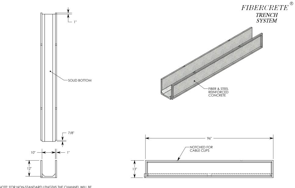
NOTE: FOR NON-STANDARD LENGTHS THE CHANNEL WILL BE DESIGNATED WITH ITS CORRESPONDING LENGTH MEASUREMENT. IE: 8810SB 32"
