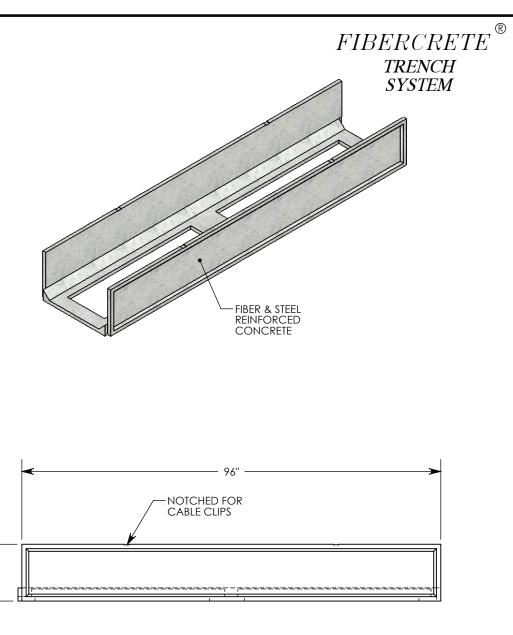
NOTE: FOR NON-STANDARD LENGTHS THE CHANNEL WILL BE SOLID BOTTOM AND DESIGNATED WITH ITS CORRESPONDING LENGTH MEASUREMENT. IE: 8820 32"
