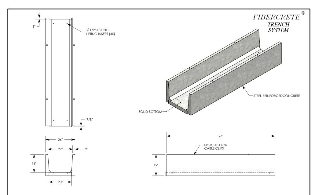
**NOTE:** FOR NON-STANDARD LENGTHS THE CHANNEL WILL BE SOLID BOTTOM AND DESIGNATED WITH ITS CORRESPONDING LENGTH MEASUREMENT. IE: 882016PTSB 32"
