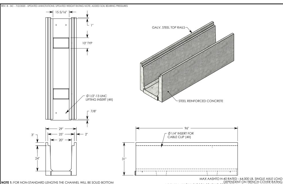
**NOTE 1:** FOR NON-STANDARD LENGTHS THE CHANNEL WILL BE SOLID BOTTOM AND DESIGNATED WITH ITS CORRESPONDING LENGTH MEASUREMENT. IE: 802024HT3 32"
