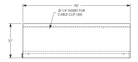
NOTE: FOR NON-STANDARD LENGTHS THE CHANNEL WILL BE DESIGNATED WITH ITS CORRESPONDING LENGTH MEASUREMENT. IE: 802024LTSB 32"
