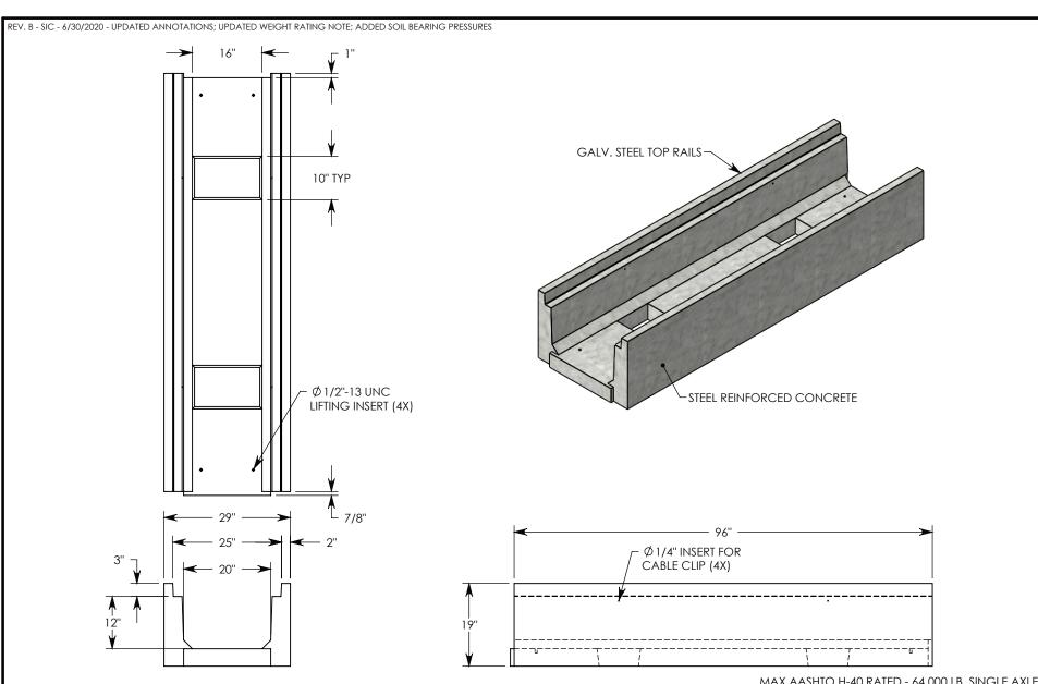
**NOTE 1:** FOR NON-STANDARD LENGTHS, THE CHANNEL WILL BE SOLID BOTTOM AND DESIGNATED WITH ITS CORRESPONDING LENGTH MEASUREMENT. IE: 8020HT3 72"
