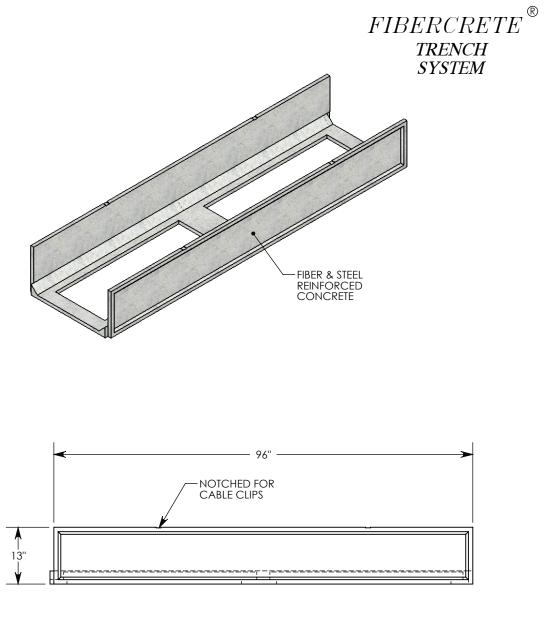
NOTE: FOR NON-STANDARD LENGTHS THE CHANNEL WILL BE SOLID BOTTOM AND DESIGNATED WITH ITS CORRESPONDING LENGTH MEASUREMENT. IE: 8824 32"
