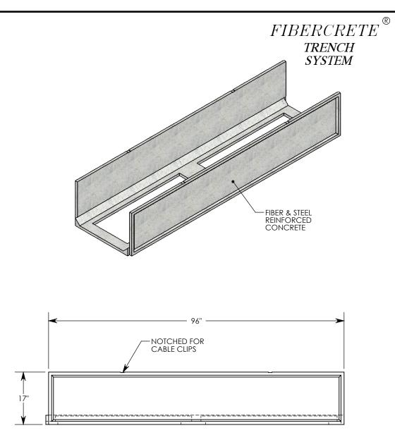
NOTE: FOR NON-STANDARD LENGTHS THE CHANNEL WILL BE SOLID BOTTOM AND DESIGNATED WITH ITS CORRESPONDING LENGTH MEASUREMENT. IE: 882416 32"
