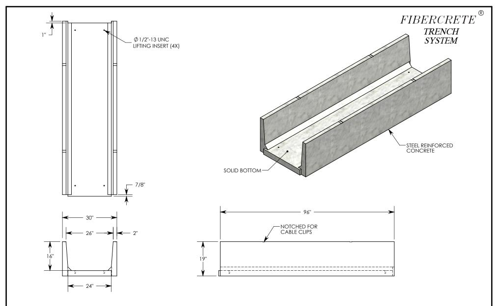
**NOTE**: FOR NON-STANDARD LENGTHS THE CHANNEL WILL BE SOLID BOTTOM AND DESIGNATED WITH ITS CORRESPONDING LENGTH MEASUREMENT. IE: 882416PTSB 32"
