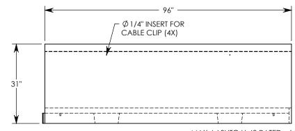
NOTE 1: FOR NON-STANDARD LENGTHS THE CHANNEL WILL BE SOLID BOTTOM AND DESIGNATED WITH ITS CORRESPONDING LENGTH MEASUREMENT. IE: 802424HT3 32" MAX AASHTO H-40 RATED - 64,000 LB. SINGLE AXLE LOAD DEPENDENT ON TRENCH COVER RATING MINIMUM ALLOWABLE SOIL BEARING PRESSURE – H-40: 3,500 PSF; H-20: 3,000 PSF
