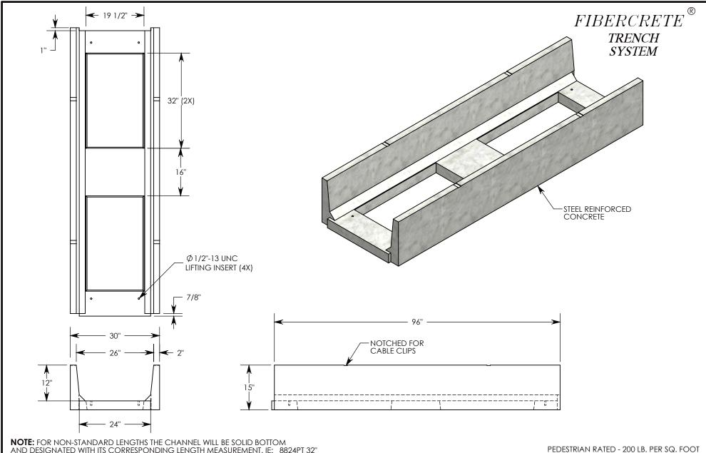
**NOTE:** FOR NON-STANDARD LENGTHS THE CHANNEL WILL BE SOLID BOTTOM AND DESIGNATED WITH ITS CORRESPONDING LENGTH MEASUREMENT. IE: 8824PT 32"
