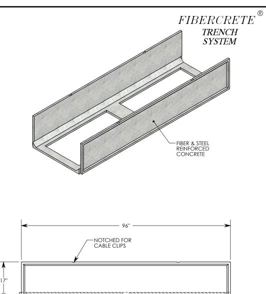
NOTE: FOR NON-STANDARD LENGTHS THE CHANNEL WILL BE SOLID BOTTOM AND DESIGNATED WITH ITS CORRESPONDING LENGTH MEASUREMENT. IE: 883016 32"
