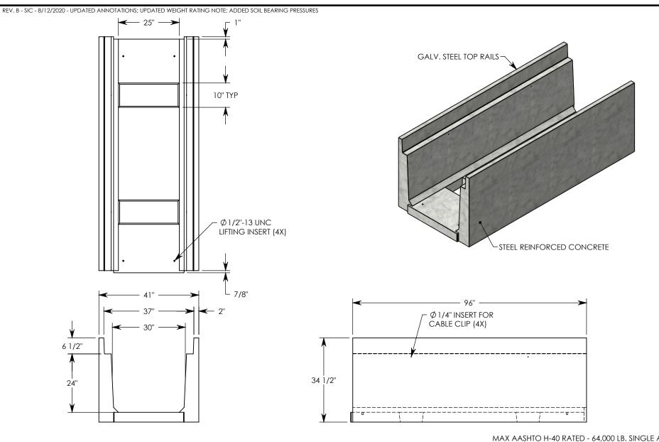
**NOTE 1:** FOR NON-STANDARD LENGTHS THE CHANNEL WILL BE SOLID BOTTOM AND DESIGNATED WITH ITS CORRESPONDING LENGTH MEASUREMENT. IE: 803024HT 32"
