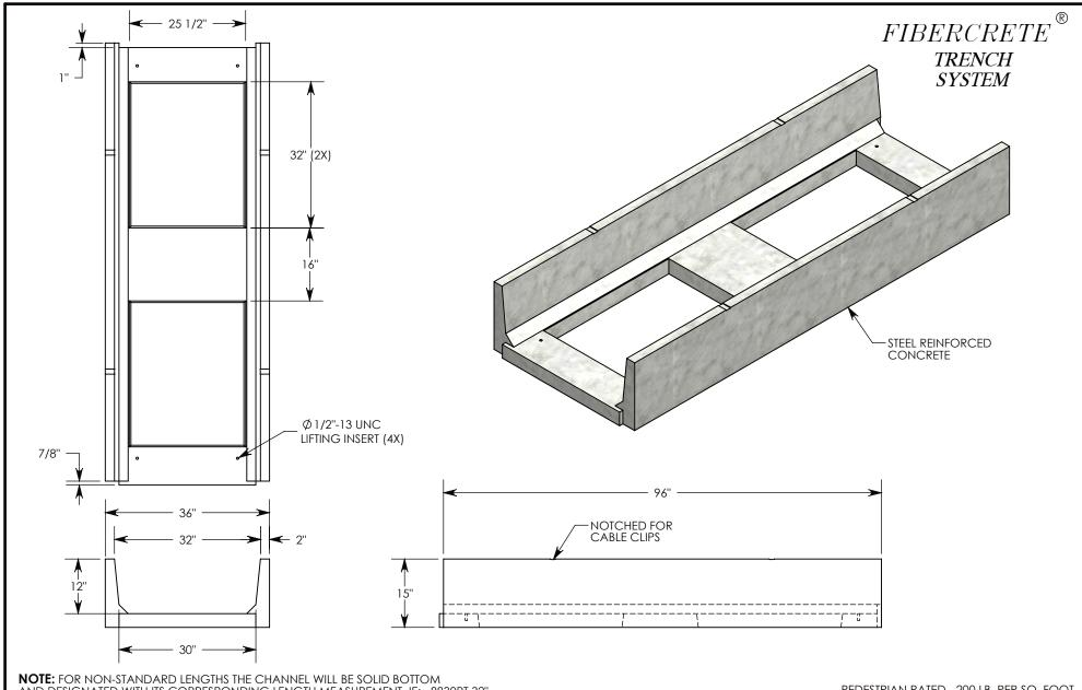
**NOTE:** FOR NON-STANDARD LENGTHS THE CHANNEL WILL BE SOLID BOTTOM AND DESIGNATED WITH ITS CORRESPONDING LENGTH MEASUREMENT. IE: 8830PT 32"
