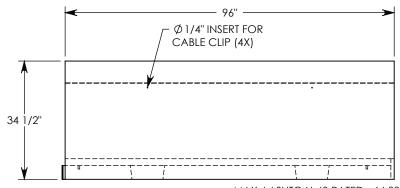
NOTE 1: FOR NON-STANDARD LENGTHS THE CHANNEL WILL BE SOLID BOTTOM AND DESIGNATED WITH ITS CORRESPONDING LENGTH MEASUREMENT. IE: 804024HT 32"
