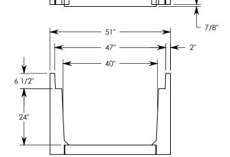
Ø 1/2"-13 UNC LIFTING INSERT (4X) GALV. STEEL TOP RAILS STEEL REINFORCED CONCRETE
