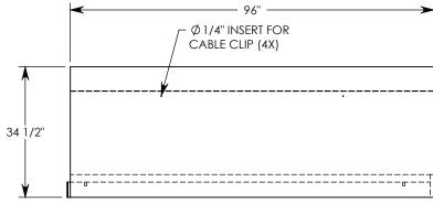
NOTE 1: FOR NON-STANDARD LENGTHS THE CHANNEL WILL BE SOLID BOTTOM AND DESIGNATED WITH ITS CORRESPONDING LENGTH MEASUREMENT. IE: 804024HT 32" MAX AASHTO H-40 RATED - 64,000 LB. SINGLE AXLE LOAD DEPENDENT ON TRENCH COVER RATING MINIMUM ALLOWABLE SOIL BEARING PRESSURE – H-40: 3,000 PSF; H-20: 3,000 PSF
