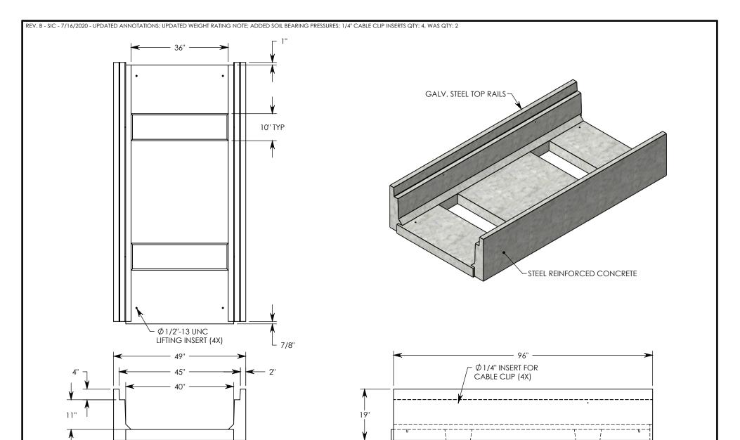
**NOTE 1:** FOR NON-STANDARD LENGTHS, THE CHANNEL WILL BE SOLID BOTTOM AND DESIGNATED WITH ITS CORRESPONDING LENGTH MEASUREMENT. IE: 8040HT4 72"
