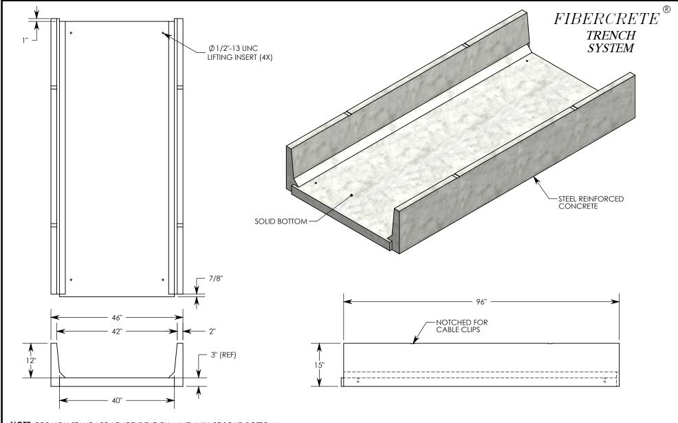
**NOTE:** FOR NON-STANDARD LENGTHS THE CHANNEL WILL BE SOLID BOTTOM AND DESIGNATED WITH ITS CORRESPONDING LENGTH MEASUREMENT. IE: 8840PTSB 32"
