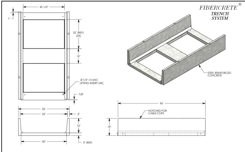
**NOTE 1:** FOR NON-STANDARD LENGTHS THE CHANNEL WILL BE SOLID BOTTOM AND DESIGNATED WITH ITS CORRESPONDING LENGTH MEASUREMENT. IE: 885016PT 32"
