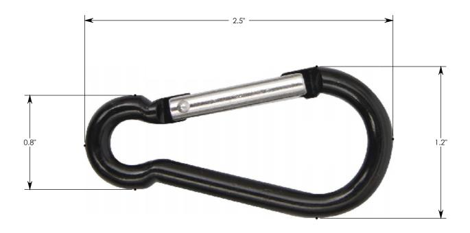
**NOTE 1:** NOT FOR USE AS LIFTING EQUIPMENT; USE ONLY FOR GUIDE POST SAFETY ROPE OR PLASTIC CHAIN **NOTE 2:** 0.8" OPENING WHEN SPRING LOADED GATE DEPRESSED
