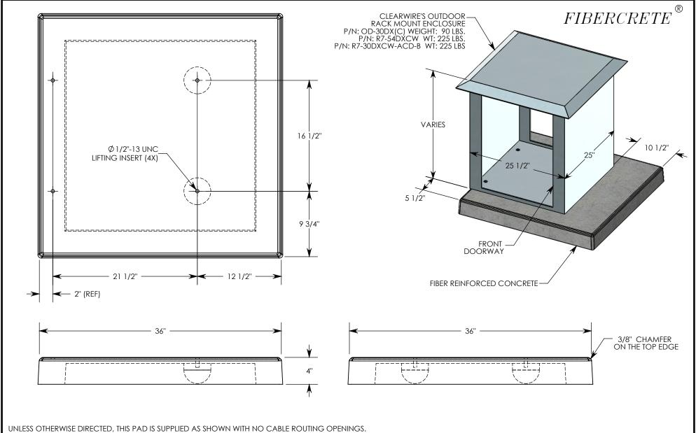
UNLESS OTHERWISE DIRECTED, THIS PAD IS SUPPLIED AS SHOWN WITH NO CABLE ROUTING OPENINGS. IF OPENINGS ARE REQUIRED, MARK-UP THIS DRAWING WITH THEIR LOCATIONS & SIZES.
