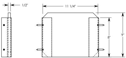
NOTE: DESIGNED TO CREATE SEPARATION IN A 18" WIDE BY 12" TALL CONCAST FHR HANDHOLE UNIT.
