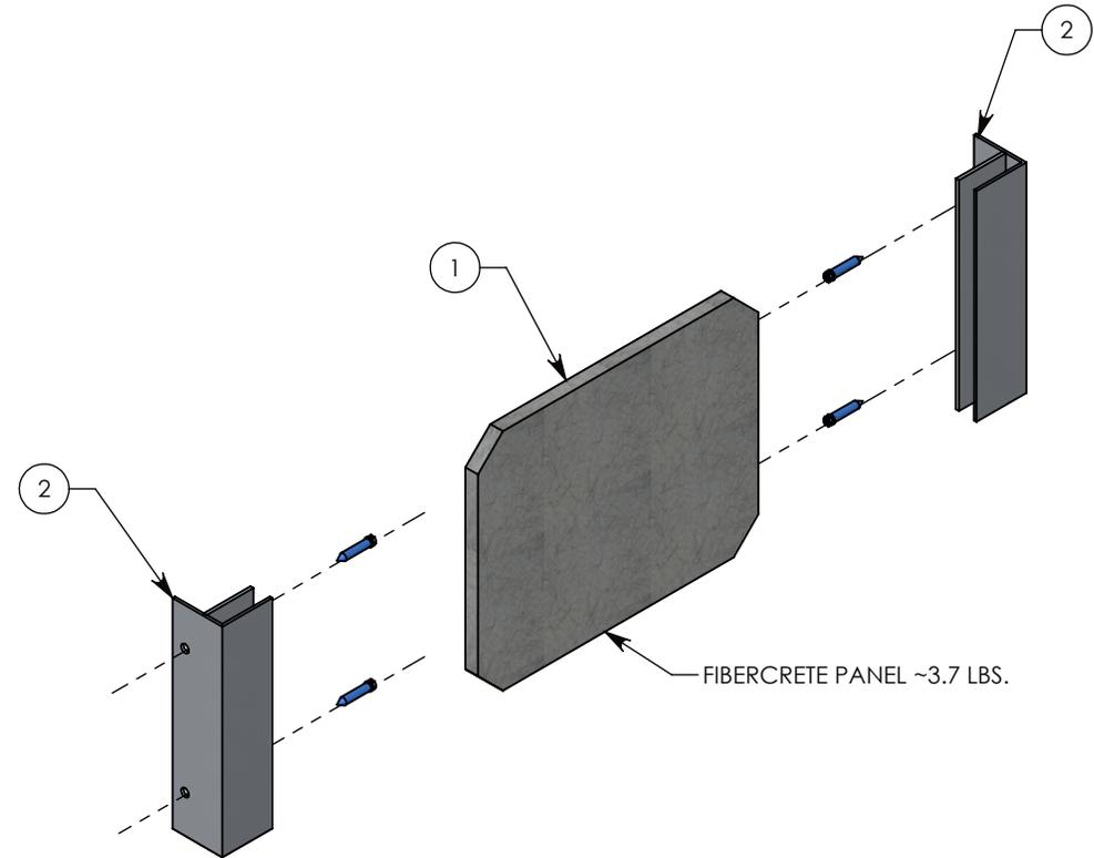
**NOTE:** DESIGNED TO CREATE SEPARATION IN A 18" WIDE BY 12" TALL CONCAST FHR HANDHOLE UNIT.
