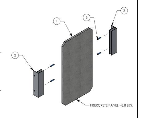
NOTE: DESIGNED TO CREATE SEPARATION IN A 18" WIDE BY 24" TALL CONCAST FHR HANDHOLE UNIT.
