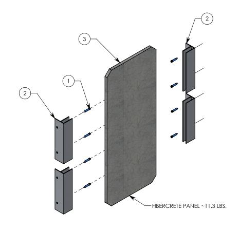
NOTE: DESIGNED TO CREATE SEPARATION IN A 18" WIDE BY 30" TALL CONCAST FHR HANDHOLE UNIT.
