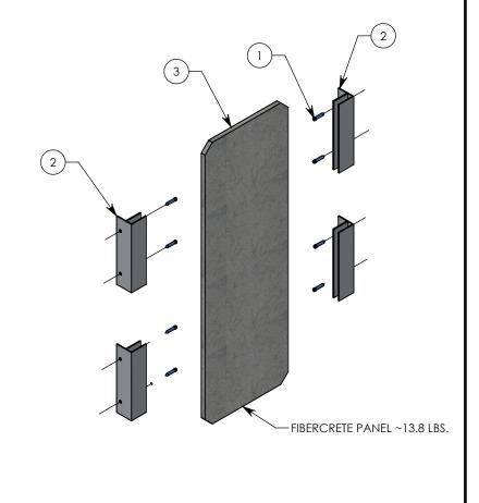
NOTE: DESIGNED TO CREATE SEPARATION IN A 18" WIDE BY 36" TALL CONCAST FHR HANDHOLE UNIT.
