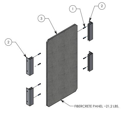
NOTE: DESIGNED TO CREATE SEPARATION IN A 24" WIDE BY 36" TALL CONCAST FHR HANDHOLE UNIT.
