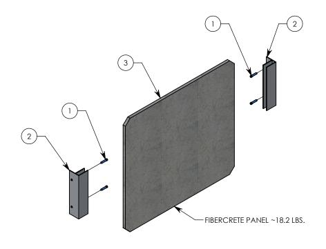
NOTE: DESIGNED TO CREATE SEPARATION IN A 30" WIDE BY 24" TALL CONCAST FHR HANDHOLE UNIT.
