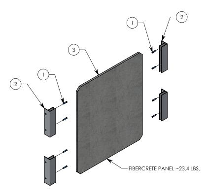
NOTE: DESIGNED TO CREATE SEPARATION IN A 30" WIDE BY 30" TALL CONCAST FHR HANDHOLE UNIT.
