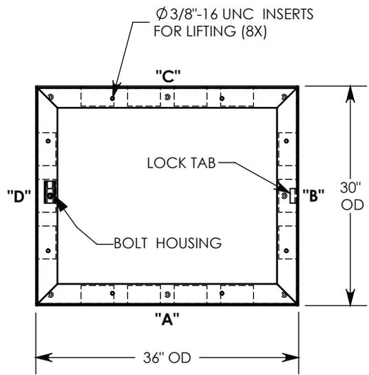
3/8-16 UNC X 1.5" LG PENTA HD BOLT (P/N: PTA.38-1.5) FOR SECURING THE COVER. BOLT HOLE IS USED FOR COVER LIFT OPERATIONS. SEE NOTE 2.
