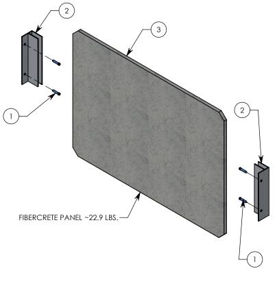
NOTE: DESIGNED TO CREATE SEPARATION IN A 36" WIDE BY 24" TALL CONCAST FHR HANDHOLE UNIT.
