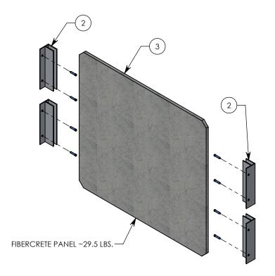
NOTE: DESIGNED TO CREATE SEPARATION IN A 36" WIDE BY 30" TALL CONCAST FHR HANDHOLE UNIT.
