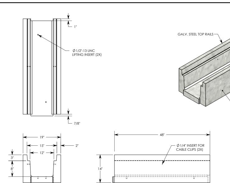
**NOTE 1:** FOR NON-STANDARD LENGTHS THE CHANNEL WILL BE SOLID BOTTOM AND DESIGNATED WITH ITS CORRESPONDING LENGTH MEASUREMENT. IE: HT1208 32"
