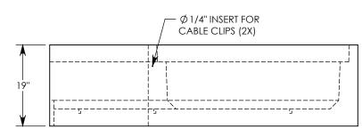
AASHTO H-20 RATED - 32,000 LB, SINGLE AXLE LOAD MINIMUM ALLOWABLE SOIL BEARING PRESSURE – 3,000 PSF
