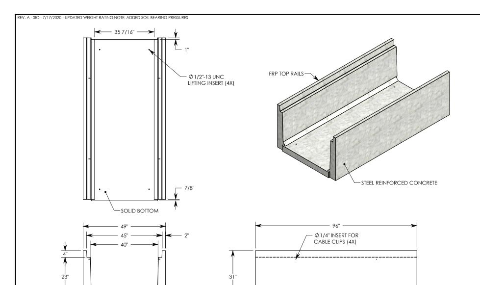
**NOTE 1:** FOR NON-STANDARD LENGTHS THE CHANNEL WILL BE SOLID BOTTOM AND DESIGNATED WITH ITS CORRESPONDING LENGTH MEASUREMENT. IE: HT4F4024 36"
