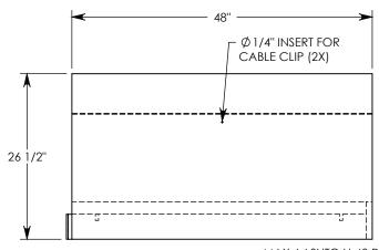
**NOTE 1:** FOR NON-STANDARD LENGTHS THE CHANNEL WILL BE SOLID BOTTOM AND DESIGNATED WITH ITS CORRESPONDING LENGTH MEASUREMENT. IE: HT6F1016 32"
