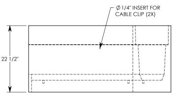
MAX AASHTO H-40 RATED - 64,000 LB. SINGLE AXLE LOAD DEPENDENT ON TRENCH COVER RATING MINIMUM ALLOWABLE SOIL BEARING PRESSURE – H-40: 3,500 PSF; H-20: 3,000 PSF
