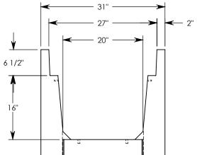
**NOTE 1:** FOR NON-STANDARD LENGTHS THE CHANNEL WILL BE SOLID BOTTOM AND DESIGNATED WITH ITS CORRESPONDING LENGTH MEASUREMENT. IE: HT6F2016 32"
