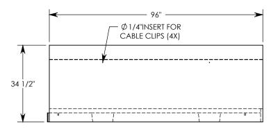
NOTE 1: FOR NON-STANDARD LENGTHS THE CHANNEL WILL BE SOLID BOTTOM AND DESIGNATED WITH ITS CORRESPONDING LENGTH MEASUREMENT. IE: HT6F2024 36" MAX AASHTO H-40 RATED - 64,000 LB. SINGLE AXLE LOAD.
