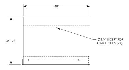
**NOTE 1:** FOR NON-STANDARD LENGTHS THE CHANNEL WILL BE SOLID BOTTOM AND DESIGNATED WITH ITS CORRESPONDING LENGTH MEASUREMENT. IE: HT6F2024 36"
