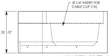
MAX AASHTO H-40 RATED - 64,000 LB. SINGLE AXLE LOAD DEPENDENT ON TRENCH COVER RATING MINIMUM ALLOWABLE SOIL BEARING PRESSURE – H-40: 3,500 PSF; H-20: 3,000 PSF
