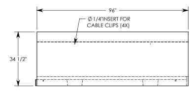
NOTE 1: FOR NON-STANDARD LENGTHS THE CHANNEL WILL BE SOLID BOTTOM AND DESIGNATED WITH ITS CORRESPONDING LENGTH MEASUREMENT. IE: HT6F2424 36" MAX AASHTO H-40 RATED - 64,000 LB. SINGLE AXLE LOAD.
